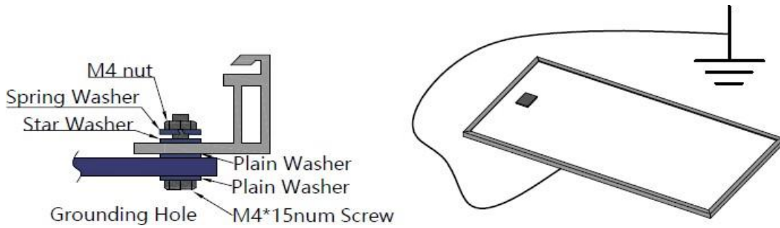
Figure 7: Ground installation of PV modules
